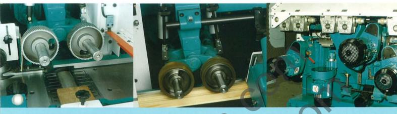
The Wadkin edge referencing system ensures the components are free of imperfections with all edges perfectly straightened. Two outfeed driven roller stations, independently adjustable, for ultimate timber control.
